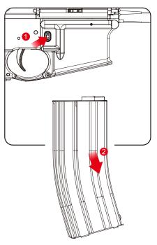
Press the magazine release button and pull the magazine downward to remove it. 按壓彈匣釋放鈕並卸除彈匣
