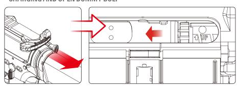
The charging handle can be pulled and the dummy bolt will lock and remain open. 向後拉動槍機拉柄,槍機飾片打開。
