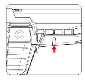
Press and hold the stock release button, then adjust the stock position. 按下槍托釋放鈕,調整槍托位置。
