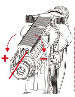
This HOP-UP system is adjusted by 3mm hex wrench. 使用3mm六角扳手調整HOP-UP系統。
