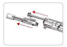
5.Remove the Bolt Assembly/卸除槍機組件 Pull back the charging handle.Take down the bolt carrier and bolt. 向後拉出槍機拉柄,並取出槍機。
