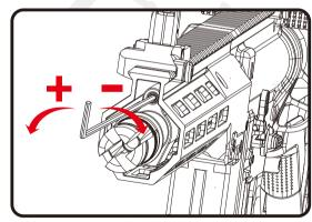
This HOP-UP system is adjusted by 3mm hex wrench. 請使用3mm六角板手調整HOP-UP。
